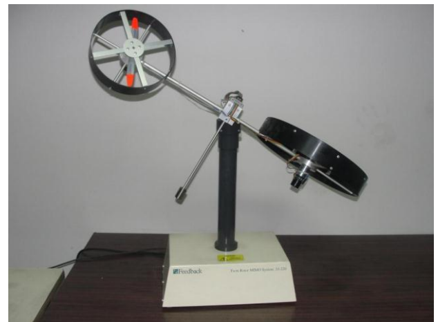
Fig.1. Twin Rotor MIMO System (TRMS).
