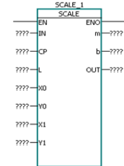
Figura 2: Bloco scale do software Ladder.
