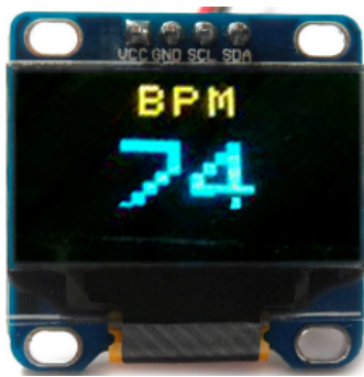
Figure 3: OLED Display SSD-1306 showing heart rate according to sensor.
